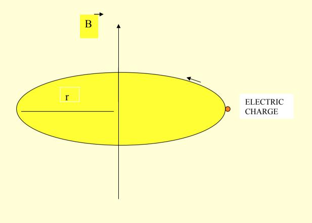
If m is the mass of the charge (q) and r the radius, the magnetic force is balanced with centrifugal force:
