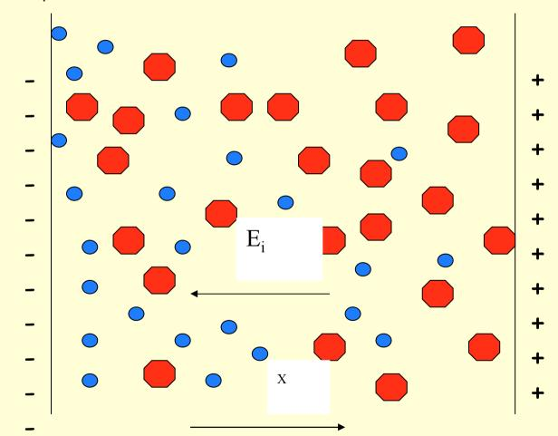
This internal electric field is:  $E=\sigma/\epsilon_{o}$ , where,  $\sigma$  is the surface density of the charge and  $\epsilon_{o}$  is dielectric permittivity of the vacuum.
