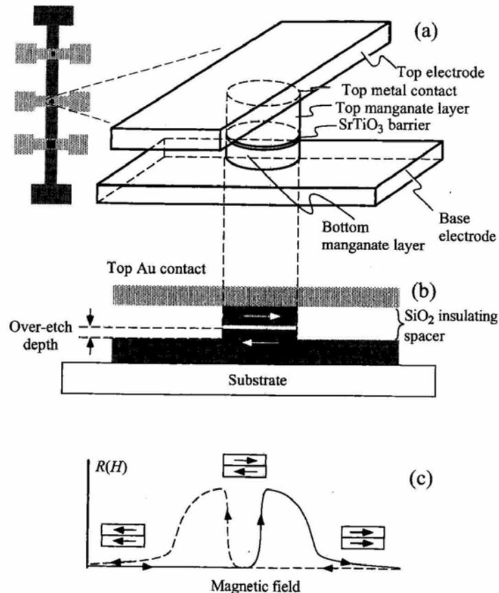
Schematic view of the LSMO-barrier-LSMO Trilayer thin film junction structure. (a) top view (b) Side view (c) junction resistance as a function of sweeping magnetic field
