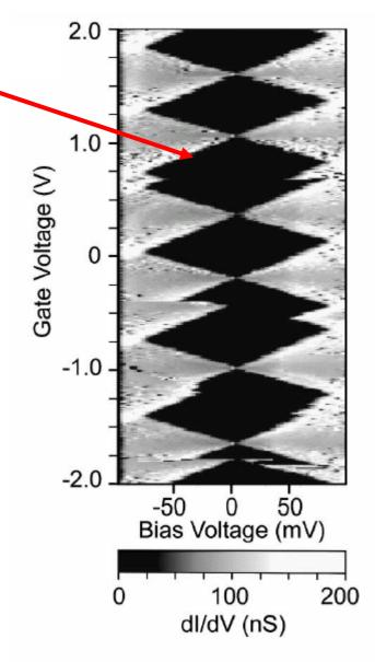
SET made with nano-particle, Bolotin et al. APL **84**, 3154 (2004)
