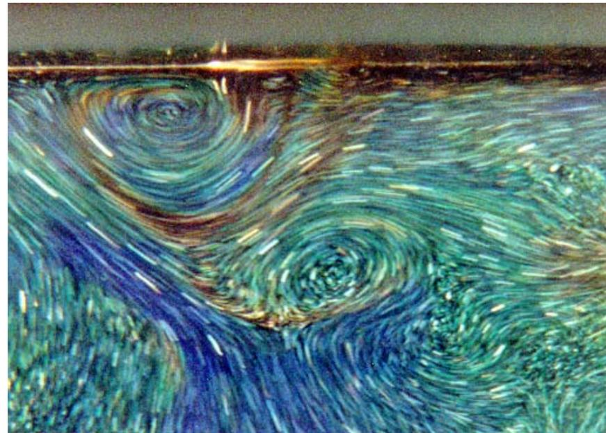
Flow visualization of turbulent thermal convection in water at  $Ra = 2.6 \times 10^9$  (6.5 cm  $\times$  4.0 cm)
