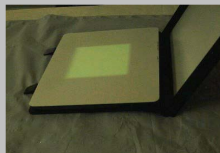
The film is exposed to both X-rays and light inside the cassette
