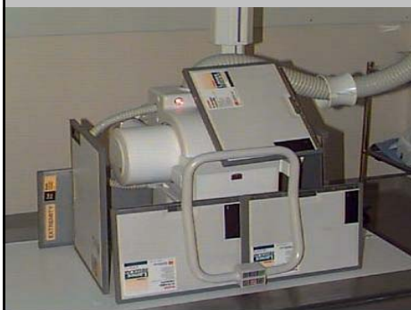
X-ray Tube Housing – Insulating Oil; Output window; Pb lining; Leakage radiation
