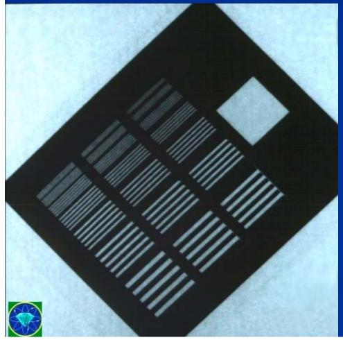
Place the test object at 45<sup>0</sup> to TV raster!
