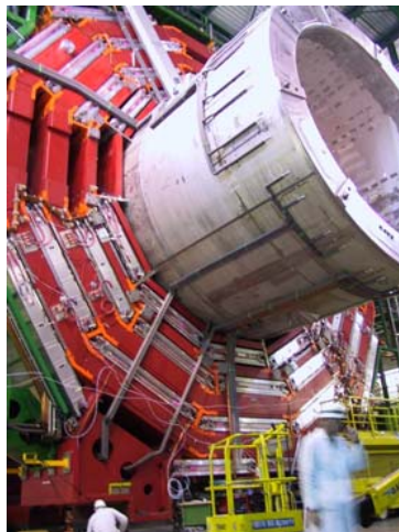
Vacuum Tank welded (Nov-Jan)
