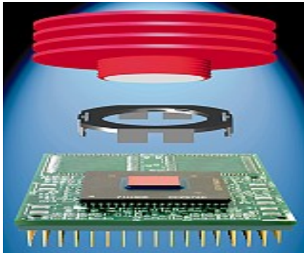
Passive heat sink
