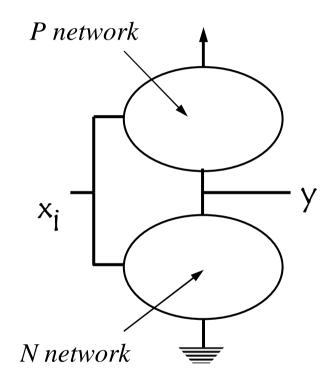
The P-network must be the dual of the N-network
