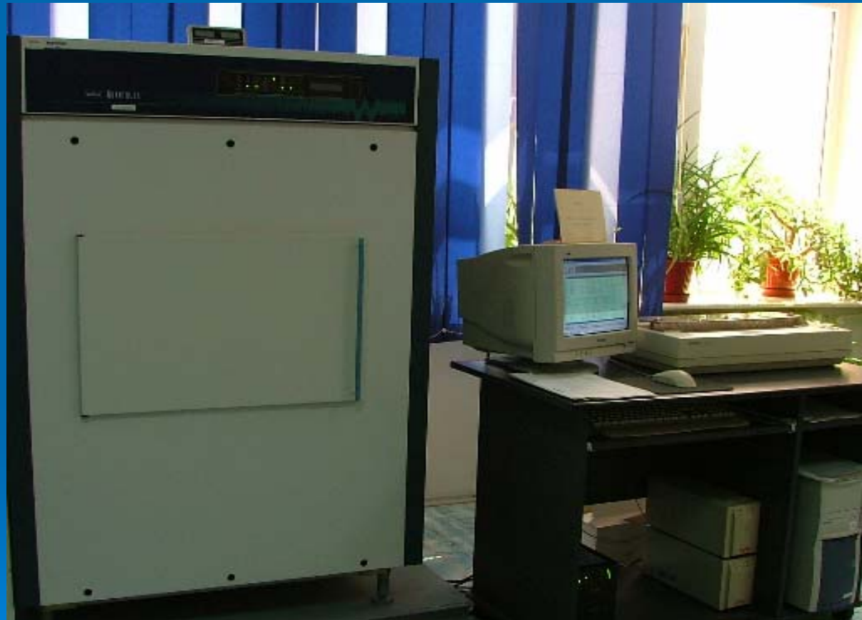
Liquid scintillation analyzer for H-3 and C-14 – Wallac, Quantulus 1220 Ultra Low Level
