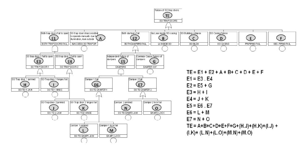
Top event (TE): Failure of SG trap door opening
