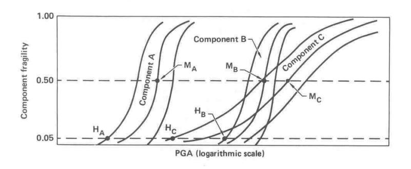
Situation – 1: Failure occurs when any one of the three systems fail Overall median capacity = median capacity of A, the weakest link.
