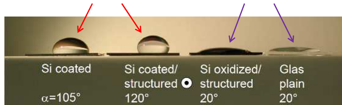
Different contact angles for water on structured (linear grating \Lambda=600\text{nm}, d=200\text{nm} ) and unstructured, plasma treated and silanated surfaces (TFS tridecafluoro-trichlorosilane)
