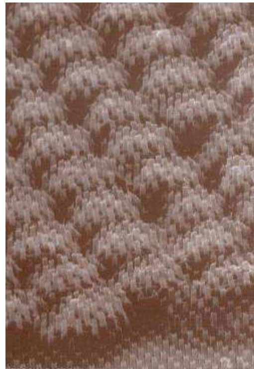
Array of pillars in PMMA with an high modulation
