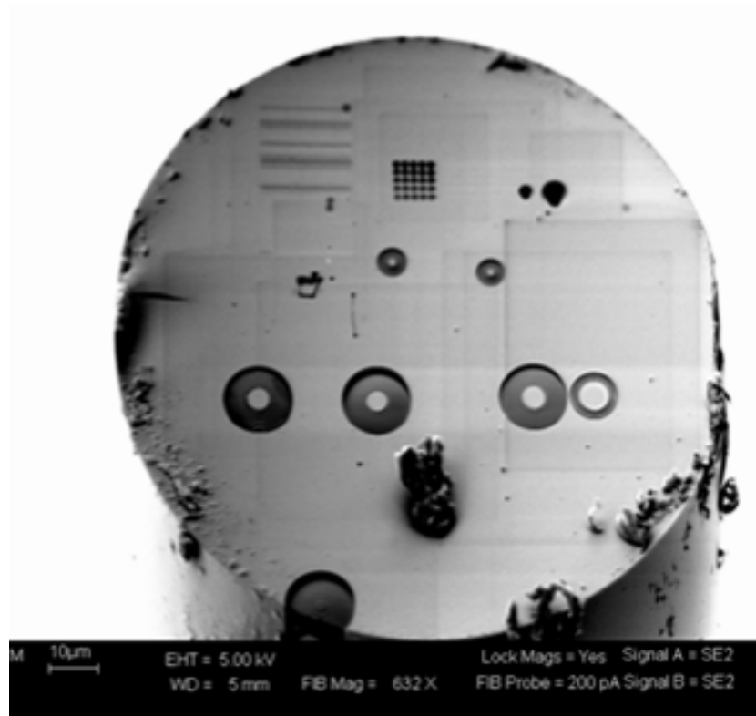
Test structures of the DOE-microlens milled on the surface by Focus Ion Beam
