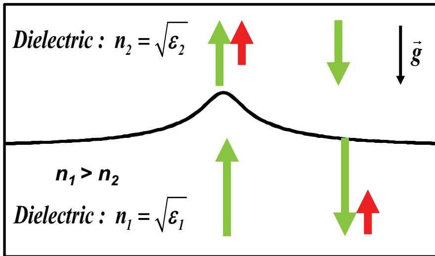
Deformation towards the optically less dense fluid
