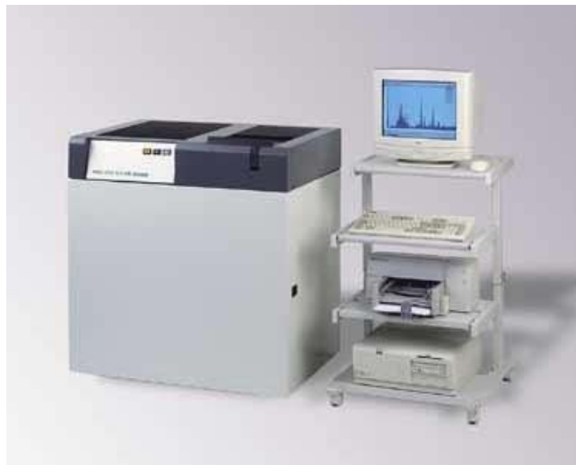
Commercial EDXR spectrometer SPECTRO 2000 (excitation using Pd-anode x-ray tube + ST and polarizers)
