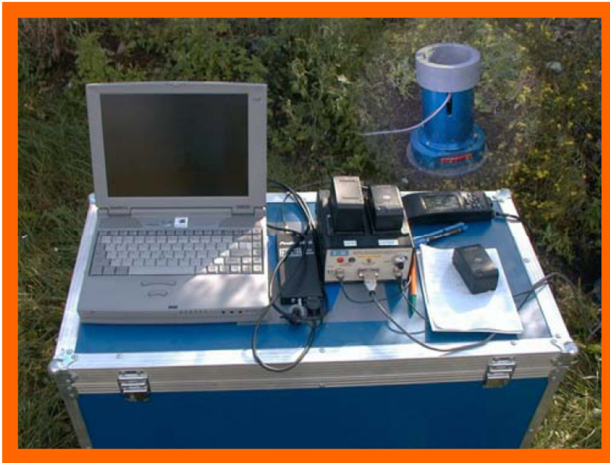
Portable spectrometer (excitation using ^{55}\text{Fe} , ^{109}\text{Cd} , ^{241}\text{Am} )
