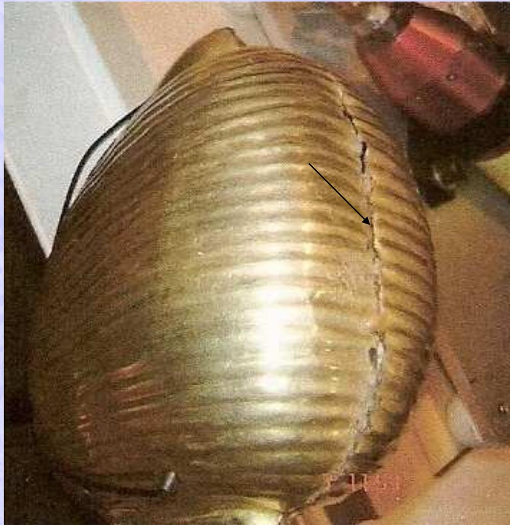
The soldering is clearly shown (arrow)
