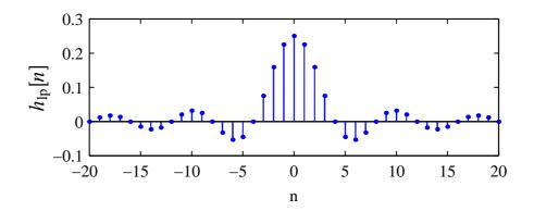
The ideal lowpass filter is noncausal, and its impulse response extends from  $-\infty < n < \infty$ . The system is therefore not computationally realisable. Also, the phase response of the ideal lowpass filter is specified to be zero — this is a problem in that causal ideal filters have nonzero phase responses.
