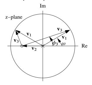
The frequency response for the single zero at different values of r and  $\theta = \pi$  is
