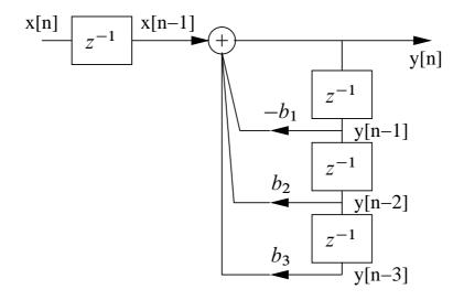
The symbol  $z^{-1}$  represents a delay of one unit of time, and the arrows represent multipliers (with the constant multiplication factors next to them). The equivalent signal flow diagram is
