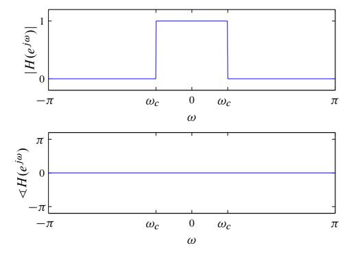
This response, as for all discrete-time signals, is periodic with period  $2\pi$ . Its impulse response (for  $-\infty < n < \infty$ ) is
