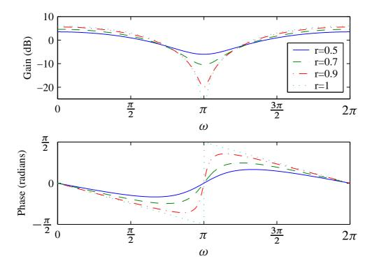
Note that the log magnitude dips more sharply as r approaches 1 (and at  $\omega = \pi$  tends to  $-\infty$  as r tends towards 1). The phase function has positive slope around  $\omega = \theta$ . This slope increases as r approaches 1, and becomes
