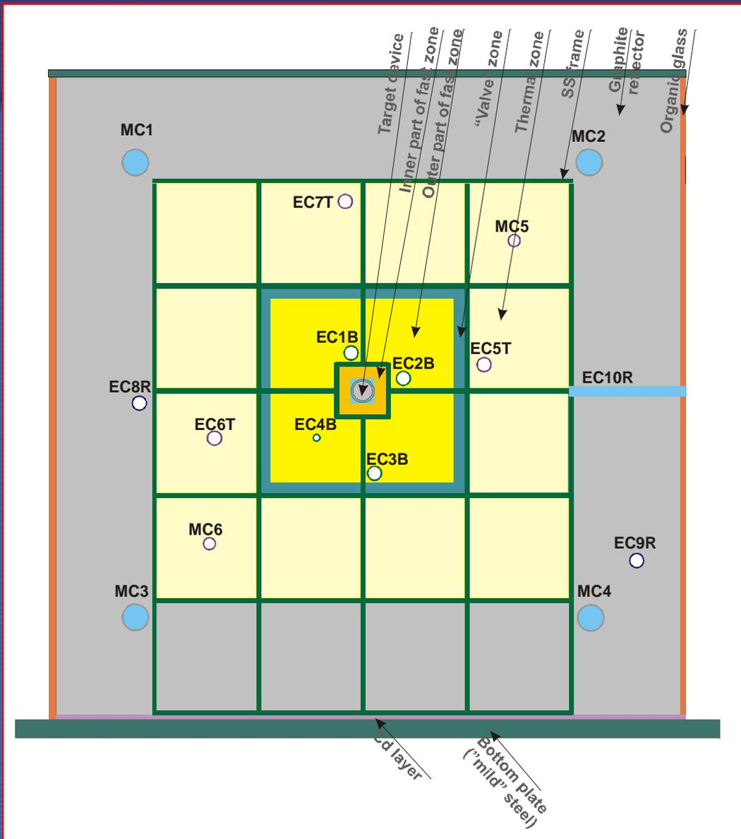
EC1B-EC4B: experimental channels in fast zone [metallic U (90%) and  $UO_2$  (36%) in Pb matrix]
