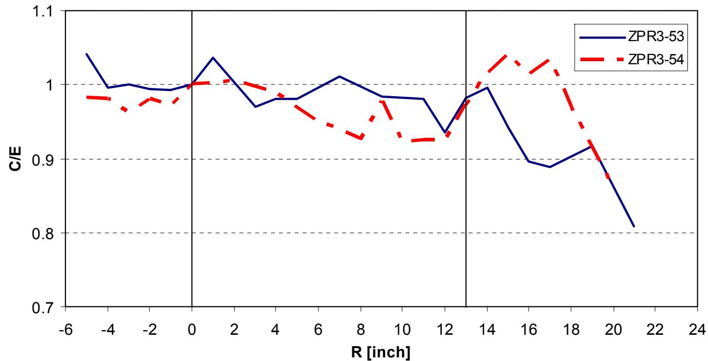
C/E in Pu239 fission rate distribution in ZPR3-53 (Blanket) and ZPR3-54 (Reflector)
