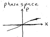
For an incoherent source (in 2D), the raysfill an area in phase space:
