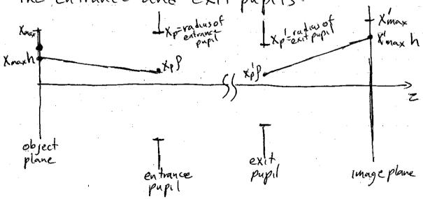
Ideally, all rays from an object point x goto the corresponding image point X'= mx (where m is the magnification), so the phase fronts in both spaces are spherical:
