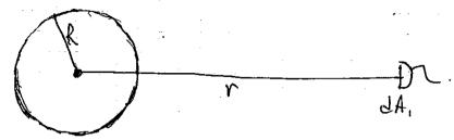
To solve this problem we use a trick, bared on the spherical symmetry of the source. Because the source is Lambertian, the radiant exitance is
