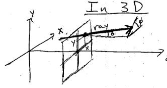
the transverse position is x = (x,y) instead of z just x. The optical momentum is  $p = (p_x, p_y)$ ,
