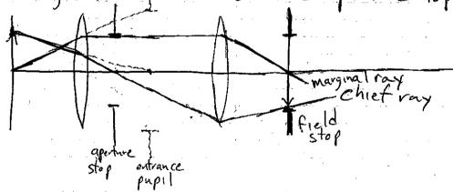
2. Marginal vay: A ray coming from the center of the object, headed for the edge of the exit pupil, and touching the edge of the aperture stop.
