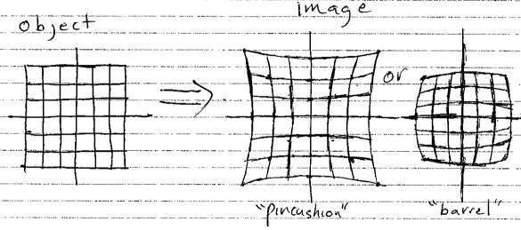
Distorsion is the only aberration that does not affect the quality of the image at the image plane, but only its shape. Novadays it can be corrected easily on the computer.
