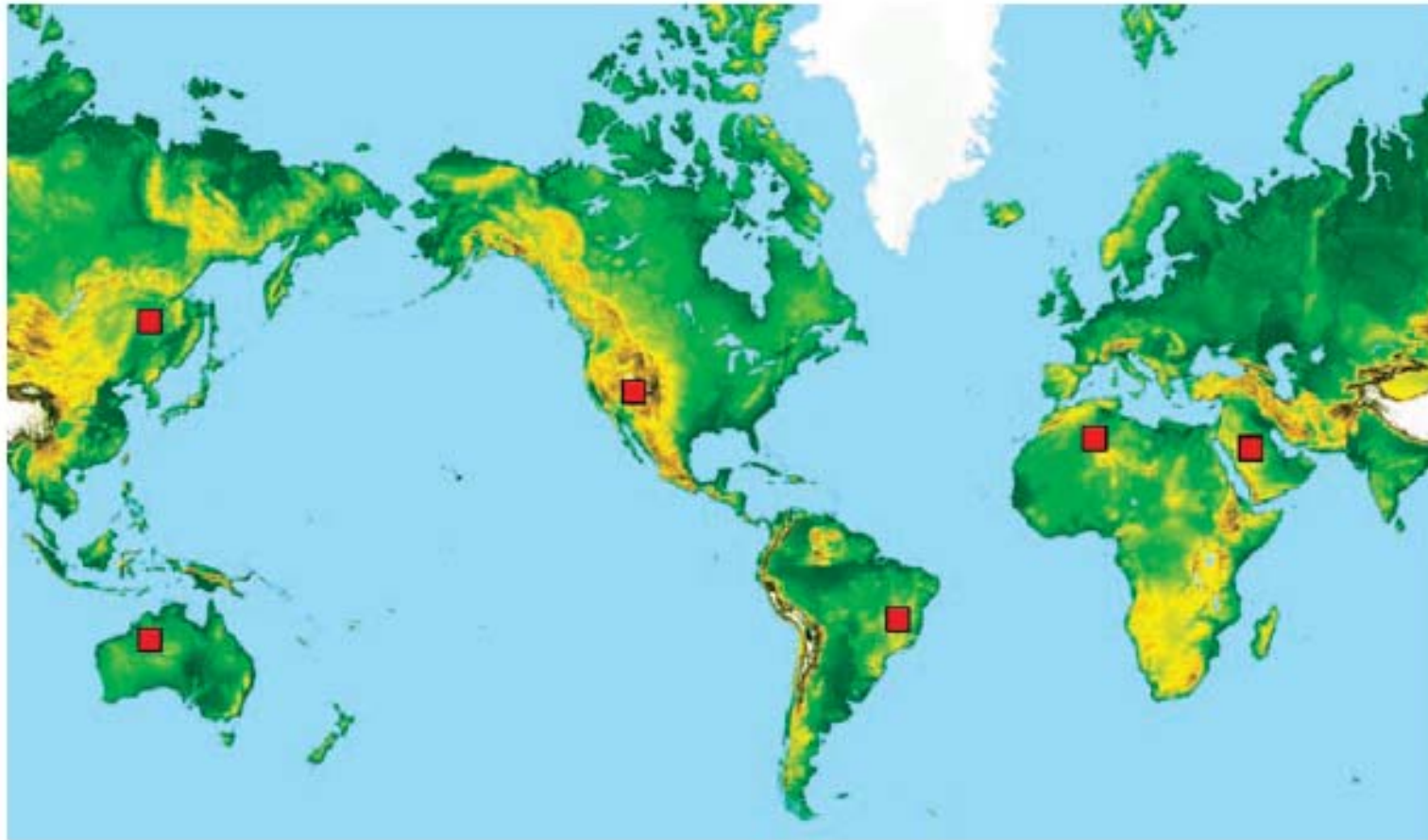
Figure 5. The production of 20 TW of power, the world's mid-century projected demand, would require covering 0.16% of Earth's land (red squares) with 10%-efficient solar panels (courtesy of Prof. Nathan Lewis, Caltech, Pasadena).
