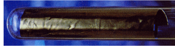
Silvery film of trans -polyacetylene
