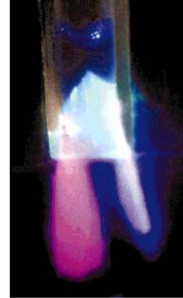
Fig. 5. The laser beams of two simultaneous random lasers in an infiltrated opal photonic crystal. The two dyes, Oxazine 670 (red) and Stilbene 140 (blue) were dissolved in methanol solution that was infiltrated into the opal. The red emission was excited at 532 nm, whereas the blue emission was excited at 355 nm using a pulsed Nd:YAG laser.
