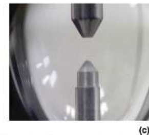
Fig. 1. (Color online) Short-arc discharge lamp. (a) Schematic [9]. (b) Typical radiance distribution from the arc of a 150 W xenon lamp, restricted to visible emission (relative to a maximum of 100% near the cathode tip) [9]. (c) Our photograph of the electrodes prior to ignition.
