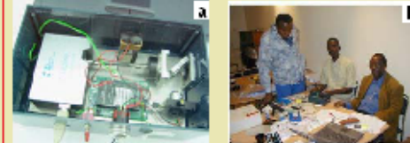
Figure 1.a: The compact fluorosensor used to induce skin fluorescence.
