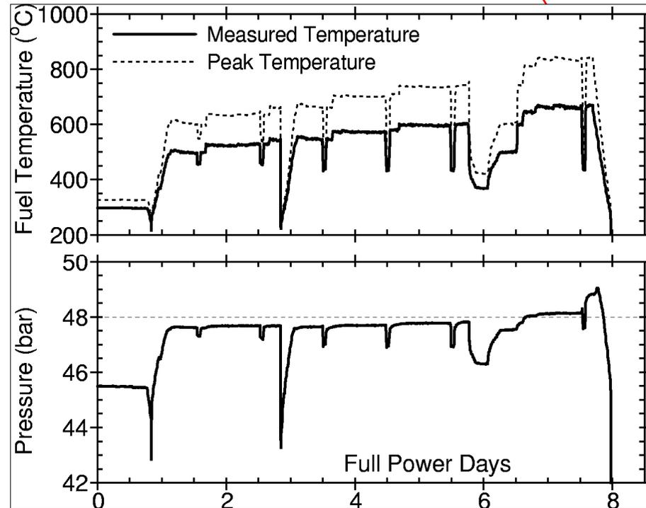
*Temperature history and measured rod pressure (fission gas release)*
