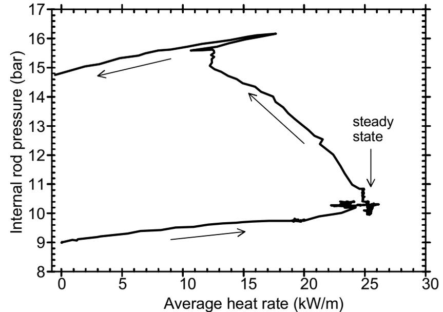
The fuel column becomes permeable after a limited power reduction. The release of the inner overpressure to the fuel rod plenum is detected then.
