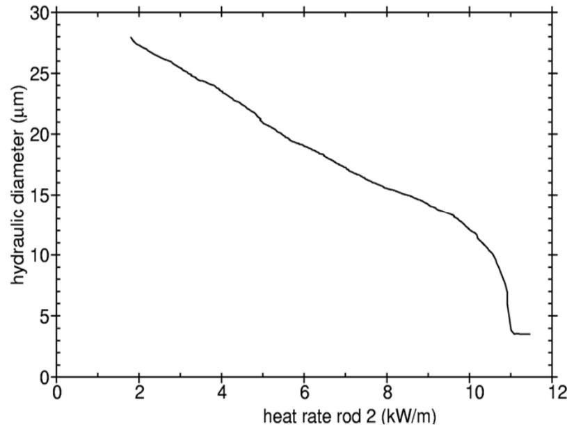
When the accommodation power level is approached, the hydraulic diameter decreases at a higher rate and the fuel column becomes very tight.
