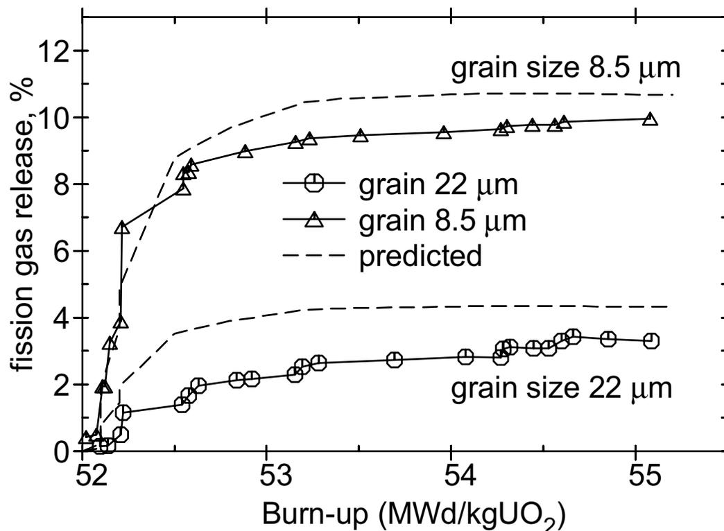
*Measured and predicted FGR for UO<sub>2</sub> fuel with different grain sizes*
