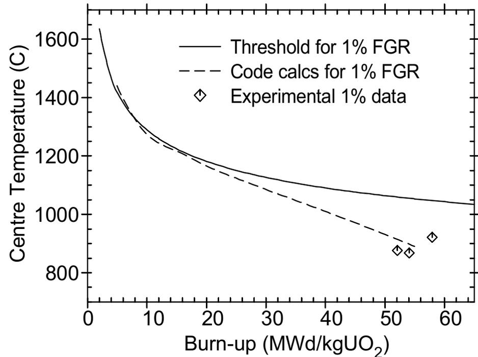
*Comparison of simple fission gas release model with empirically derived release threshold and experimental data at high burnup*
