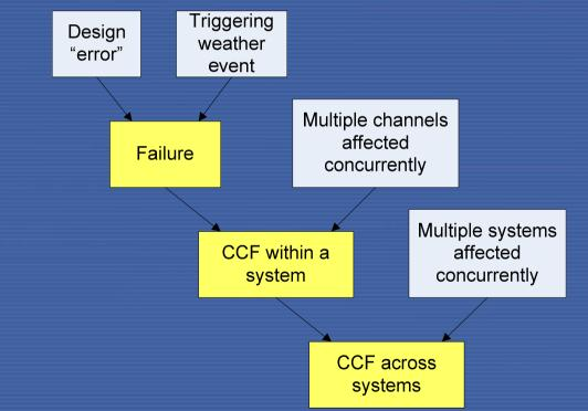
External effect beyond design basis, for which redundancy and single failure criteria were not followed.
