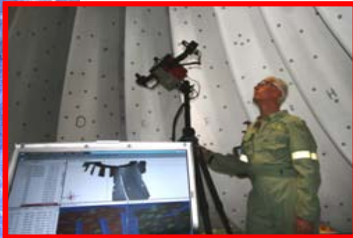
Runner geometry measurement on site
