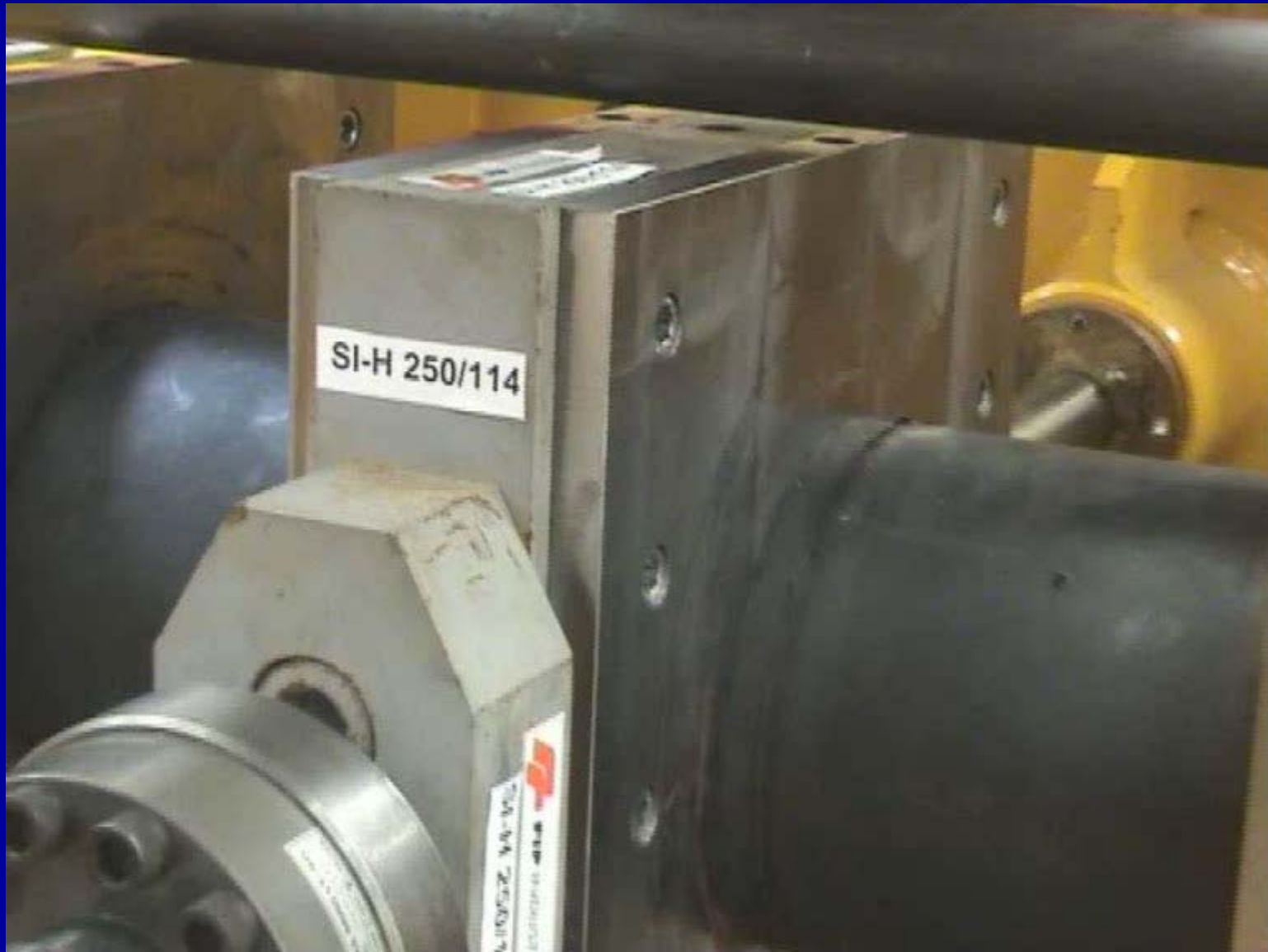
Rubber bearings: type test at FIP Industriale Laboratories & on-site test of an isolated building at Solarino (Syracuse)
