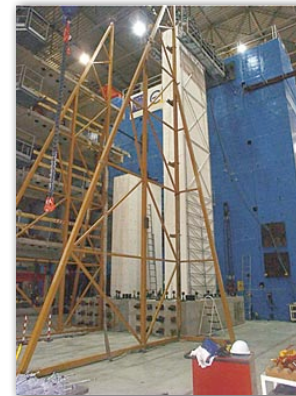
(a) physical piers in the lab, (b) schematic representation (c) workstations running the PSD algorithm and controlling the test
