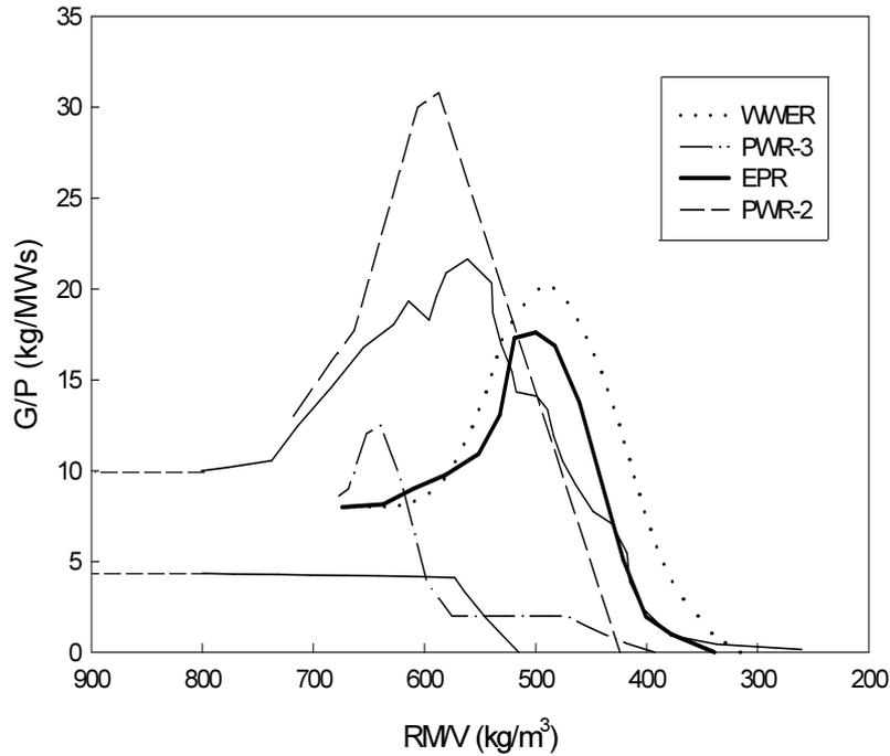
FIG.5 – Evaluation of the NCP for PWR-1, PWR-2, WWER-1000 and EPR NPP (Tab. 2) by using the NCFM.
