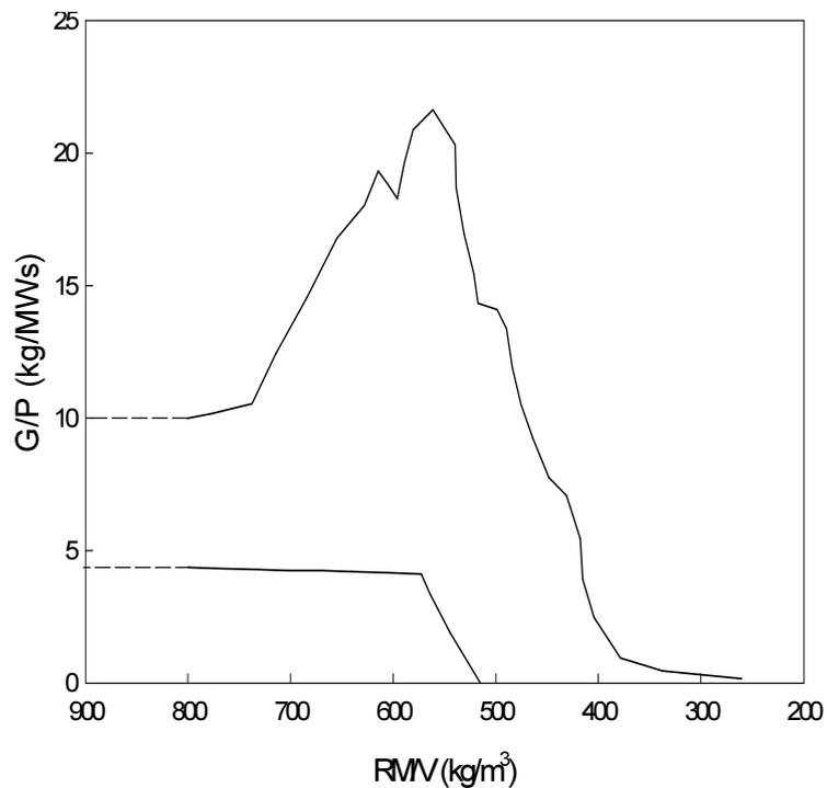
FIG. 4. – Natural Circulation Flow Map derived from the envelope of measured NC flow-rates curves in PWR simulator.
