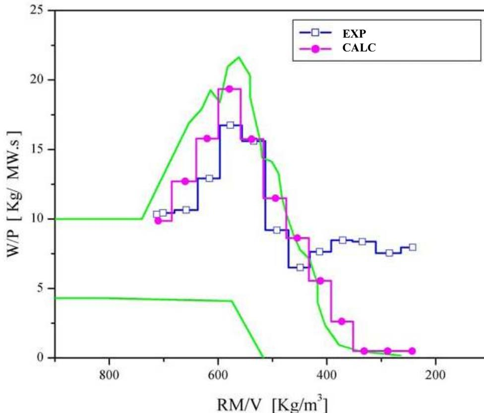
FIG. 9. Evaluation of the NCP for PSB-VVER ITF by using the NCFM: experimental data and results of calculations are reported.
