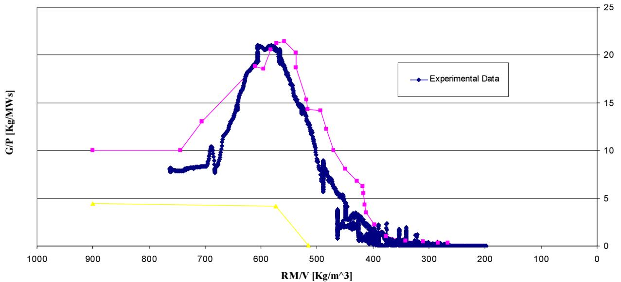
FIG. 10. Evaluation of the NCP for PKL-III ITF by using the NCFM: experimental data are reported.
