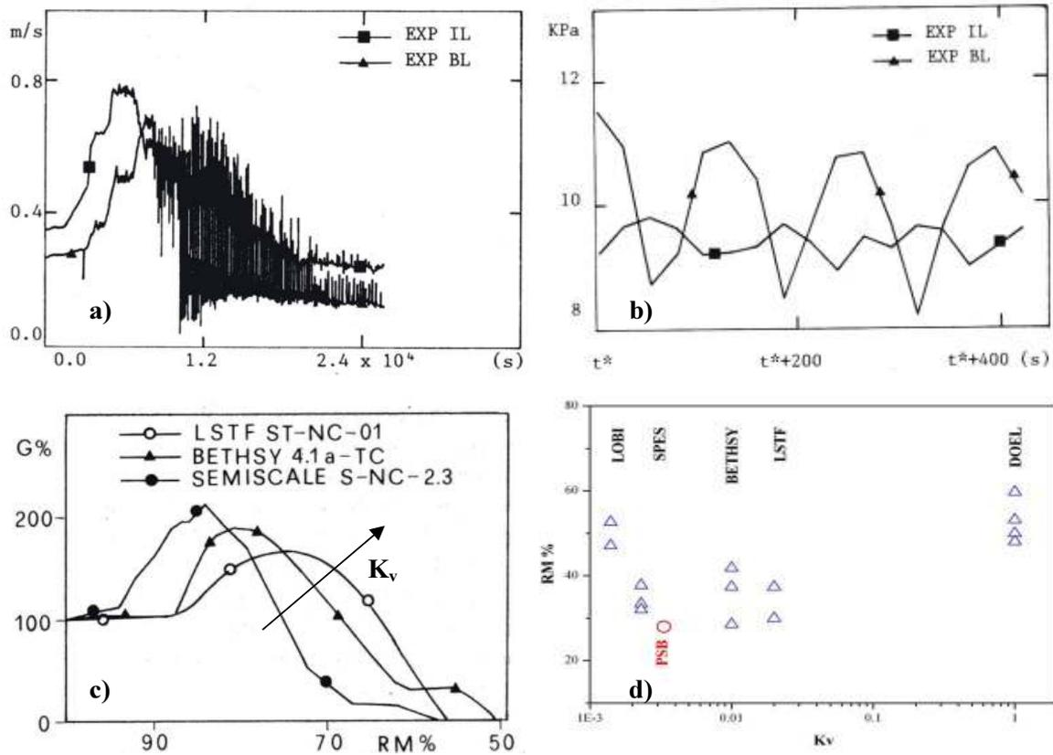
FIG. 2 – Natural circulation phenomenology in PWR: a) fluid velocity in hot leg and cold leg; b) differential pressure at inlet of steam generators; c) effect of volume scaling upon the NC curve; d) dry-out occurrence as a function of mass inventory in different PWR systems (ITF and NPP). In relation to PSB, see additional remarks in section 4.2.
