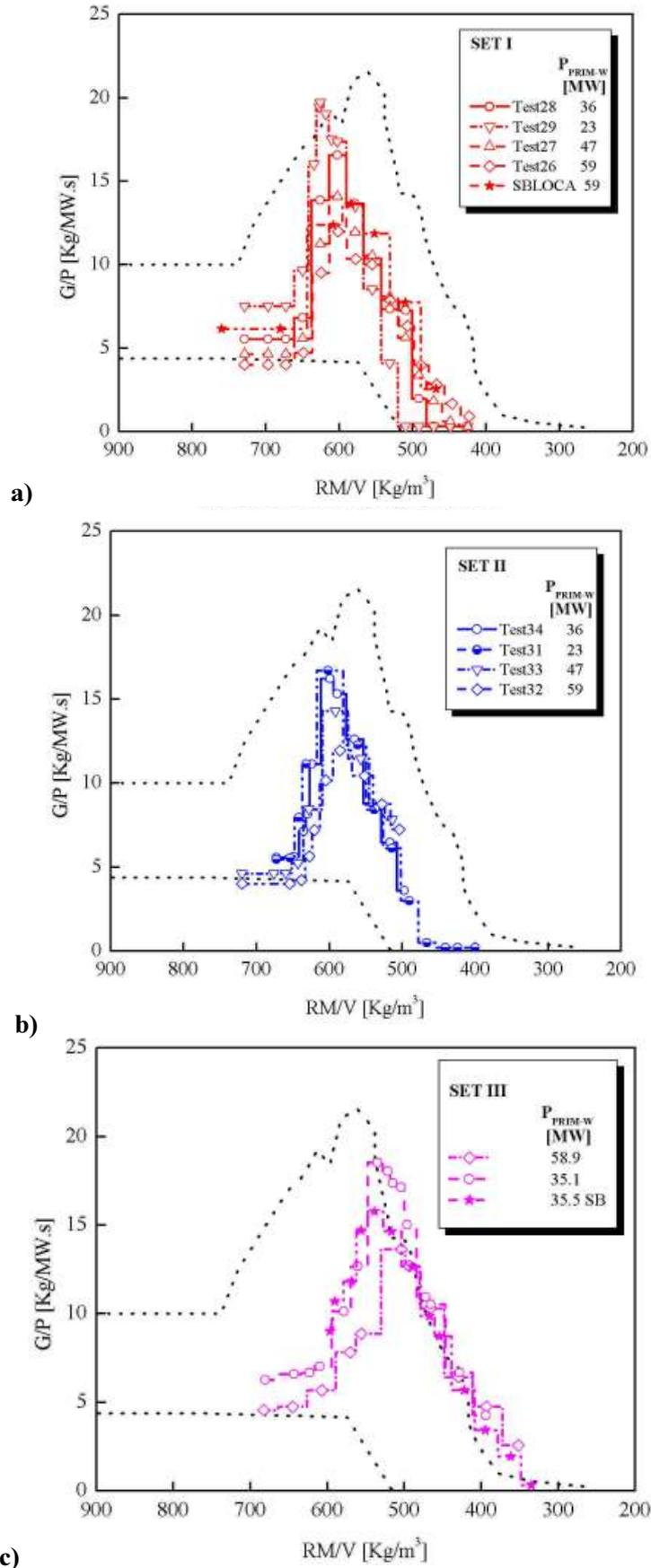
FIG. 8. Evaluation of the NCP for Atucha-1 NPP (Tab. 5) by using the NCFM: results from three different nodalizations, a) SET-I, b) SET- II and c) SET- III.
