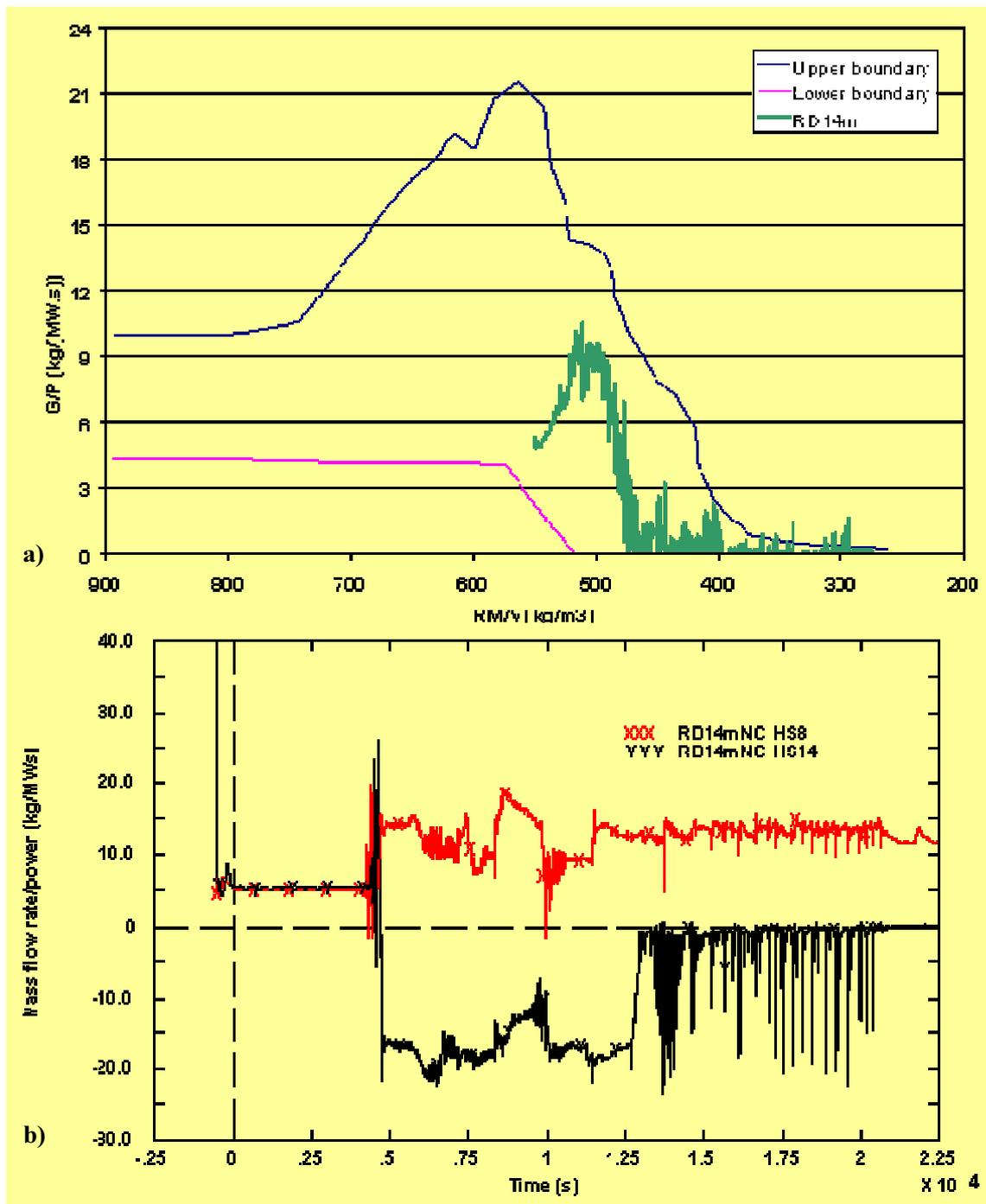
FIG. 11. Evaluation of the NCP for RD-14m ITF by using the NCFM, calculated data are reported: a) NCFM with calculated NCP; b) time trend, during the calculated NC scenario of mass flow-rates across two of the horizontal channels of the ITF.
