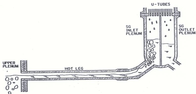
Figure 7: Schematic of liquid distribution during reflux condensation in PWRs
