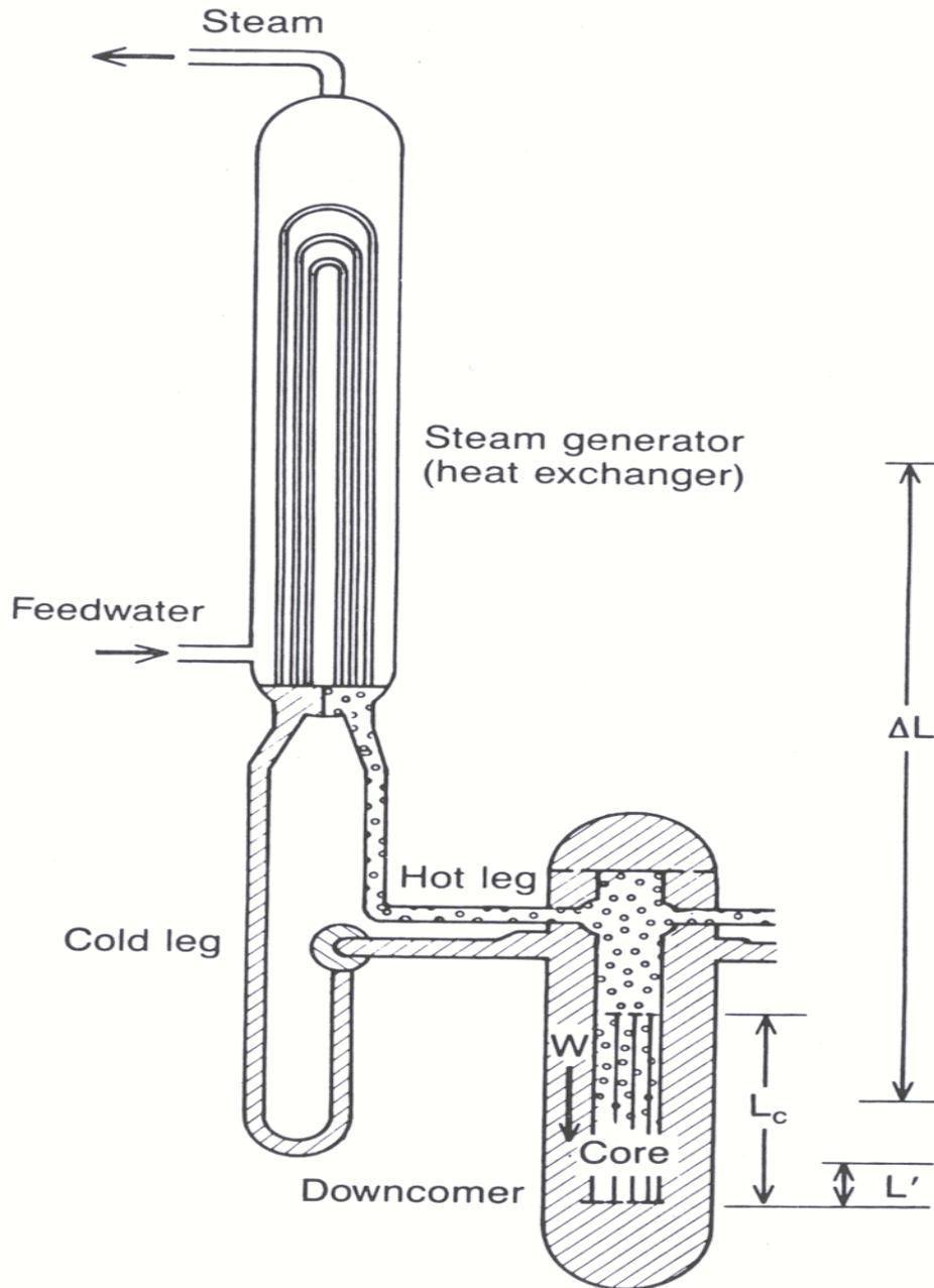
Figure 1: Schematic of a typical PWR system and elevations
