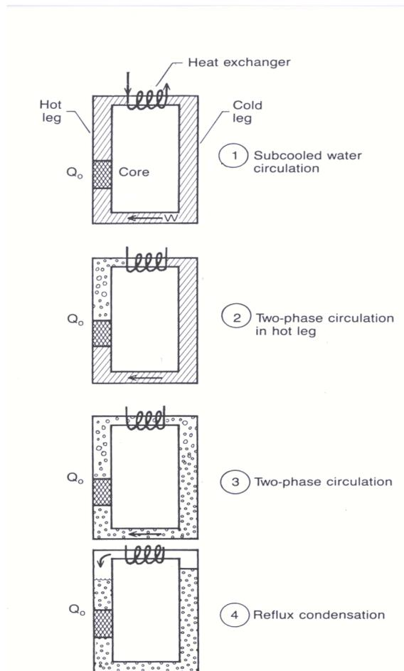
Figure 6: Different modes of natural circulation cooling in a PWR
