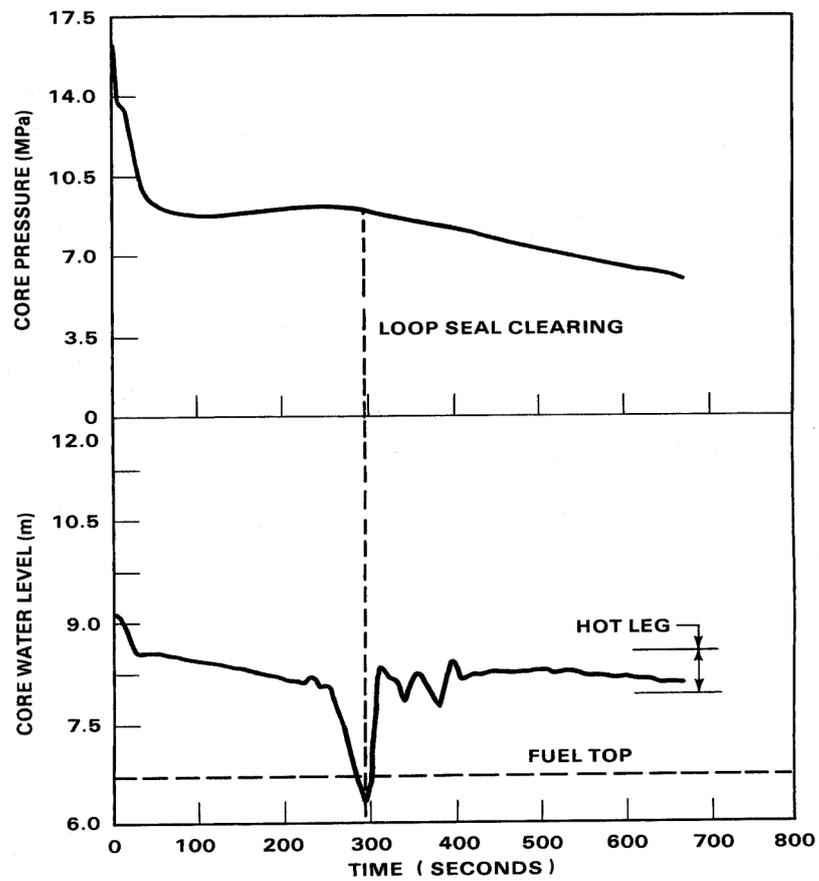
Figure 5: Typical transients of the primary system pressure and reactor vessel water level following a small break LOCA at the cold leg in a PWR
