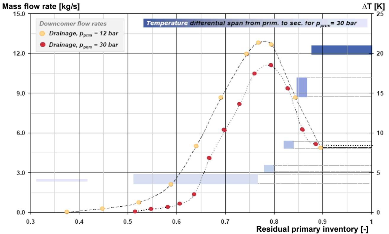
Figure 8: Downcomer mass flow rates during drainage and primary to secondary temperature differences as functions of residual primary mass inventory for PKL-III test facility (Power = 600 kW,  $P_{prim} = 12$  and 30 bar) [6]
