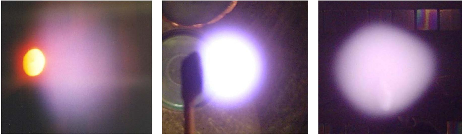
**Photos from the Innsbruck DP-machine with  $n_{pl} \cong 10^{15}-10^{16} \text{ m}^{-3}$  and  $p \cong 0,5 \text{ Pa}$**
