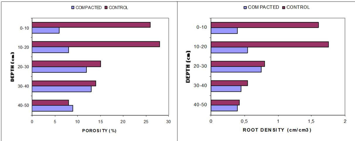
Fig. 6 – Effects of soil compaction, caused by wheel traffic of machines in a peach orchard, on soil porosity expressed as a percentage of the area occupied by pores larger than 50  $\mu\text{m}$  per thin section (on the left) and on root density expressed as root length/cm<sup>3</sup> (right).
