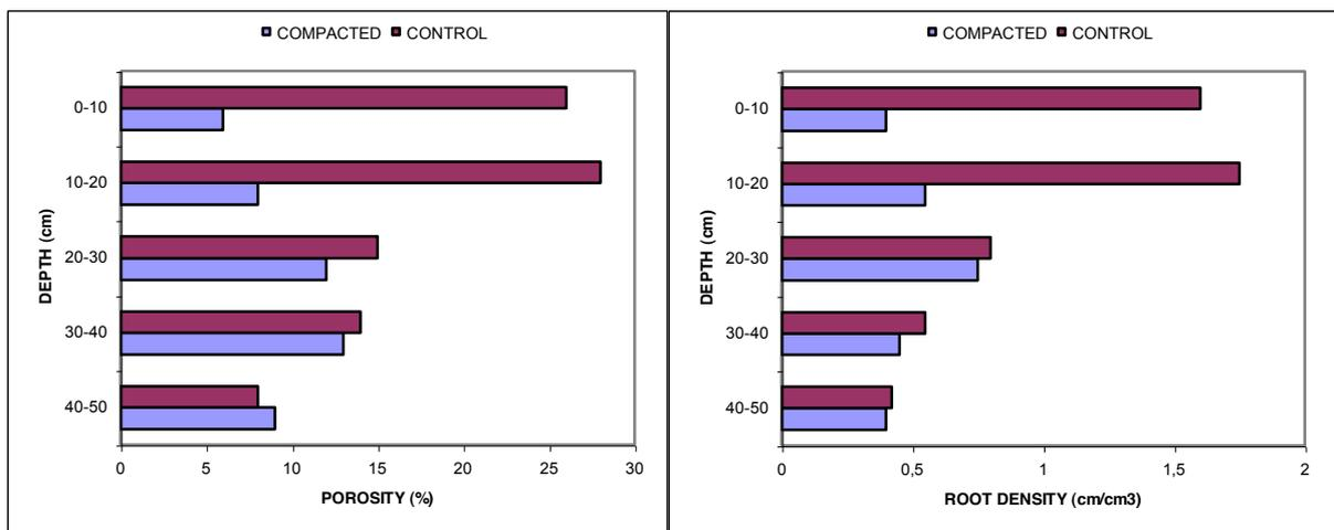
Fig. 7 - Effects of soil compaction, caused by wheel traffic of machines in a peach orchard, on soil porosity expressed as a percentage of area occupied by pores larger than 50  $\mu\text{m}$  per thin section (on the left) and on root density expressed as root length/cm<sup>3</sup> (right).
