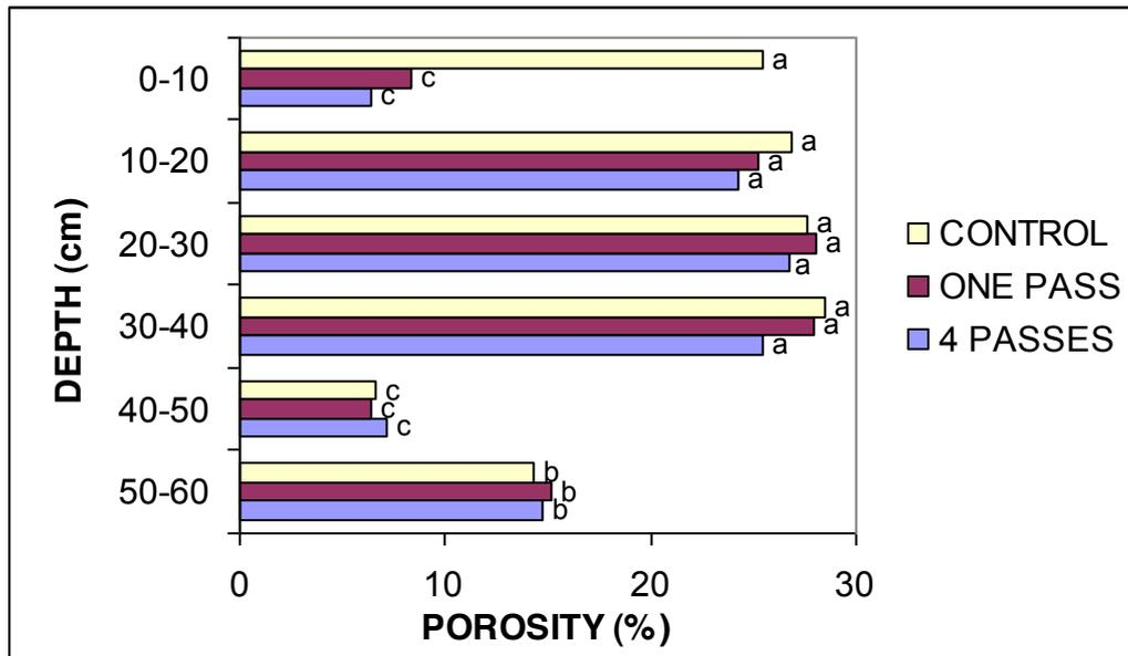
Fig. 1 – Effects of soil compaction, caused by one and four passes of tractors, on soil porosity expressed as a percentage of area occupied by pores larger than  $50 \mu\text{m}$  per thin section. Mean of six replications. Values followed by the same letter are not significantly different at the 0.05 level employing Duncan’s Multiple Range Test.
