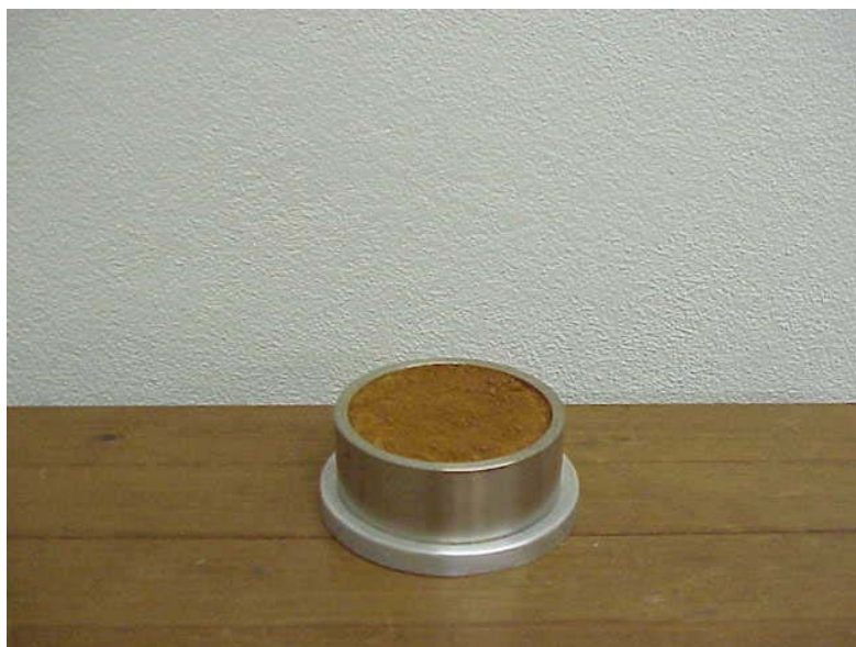
Figure 2: Undisturbed soil sample and the aluminum ring.
