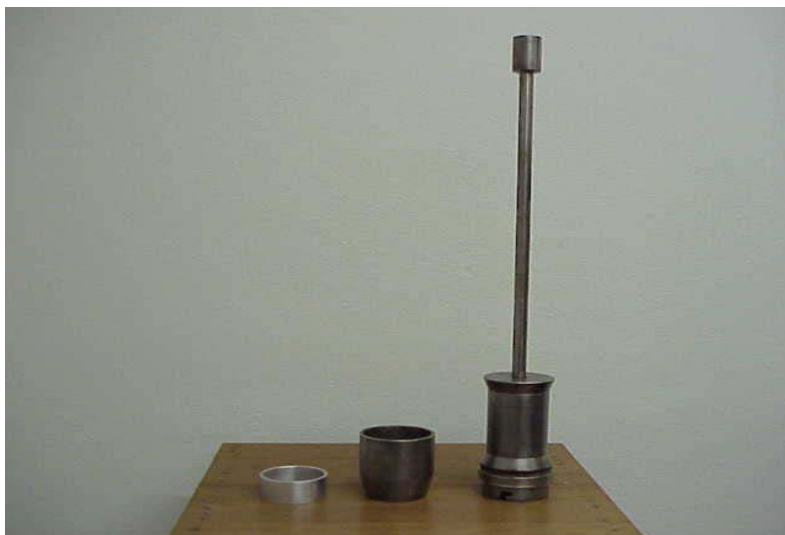
Figure 1: Uhland soil sampler and aluminum ring.
