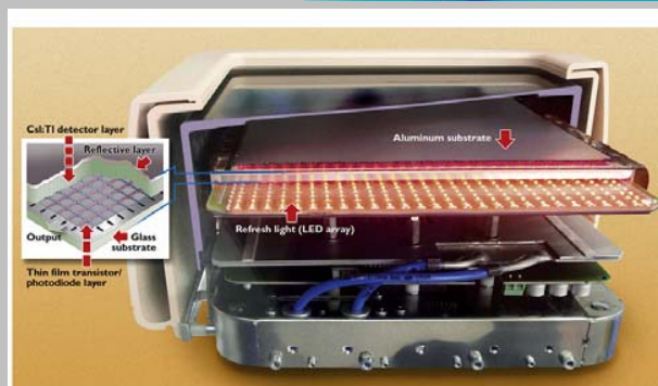
2 - Cross section through a flat panel detector. Source: Cowen et al, 2008
