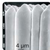
Figure 5: (a) Spectral emission of the CsI:TI crystal matches the spectral response of a-Si:H photodiodes using in x-ray indirect detection systems [9]. (b) electron micrograph of the needle shaped CsI:TI scintillation crystal [10].
