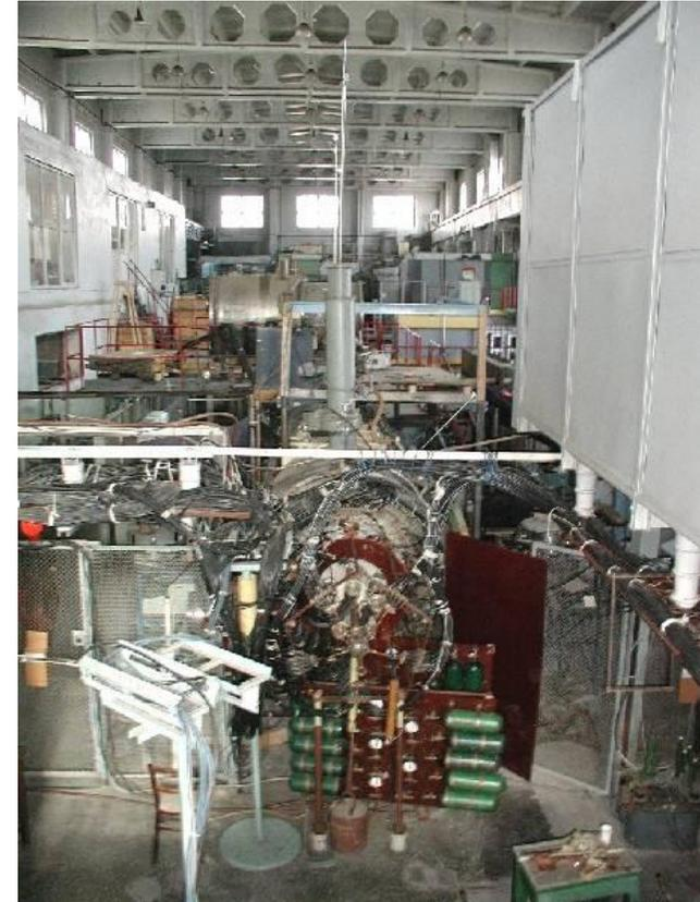
Maximal energy of capacitors supplying the main discharge WC is 2.25 MJ (plus 2 MJ for auxiliary systems ). Main results were obtained with capacitor voltage of the main discharge up to 15 kV ( $W \approx 0.8$  MJ). The maximum discharge voltage achieved 12 kV and maximum discharge current - 750 kA.
