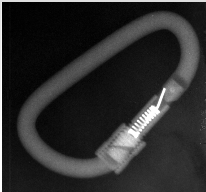
Hard x-ray introspective image of a metallic climbing carabiner.
