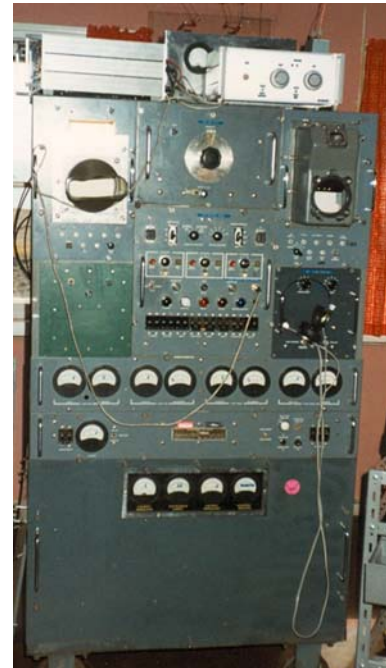
Figure 5.1.1. An old (C4) ionosonde (Narsarsuaq, Greenland ). Photo: DMI.
