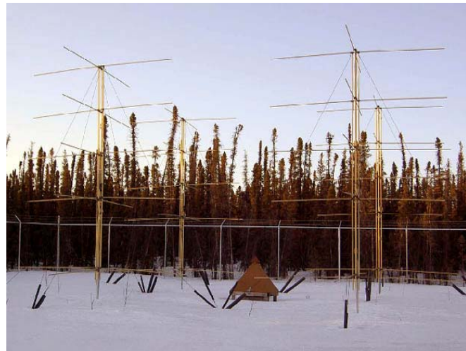
Figure 5.4.4. 4-Yagi HAARP riometer antenna system. Photo from HAARP web site.
