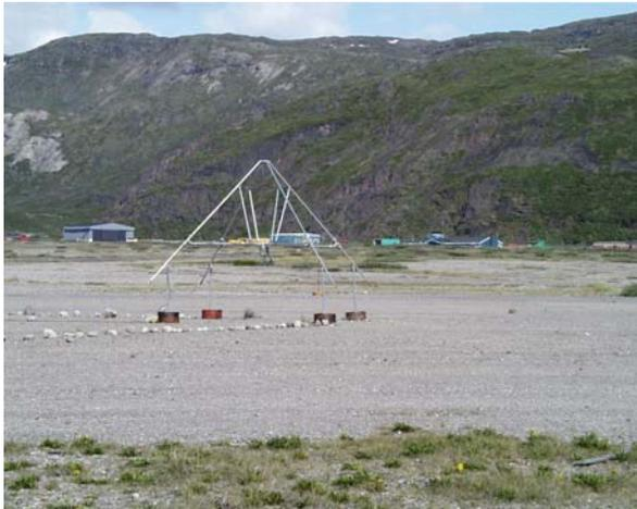
Upper left: Univ. Lowell Digisonde. Lower left: Receiver antenna. Above. Digisonde installation in Narsarsuaq. Note the tower that carries the transmitting delta antenna.
