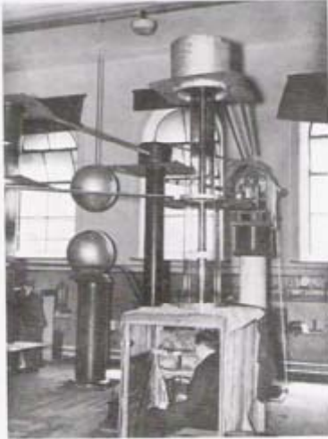
The Cockcroft-Walton accelerator which was used for the first nuclear reaction experiment in 1932. Courtesy of the University of Cambridge, Cavendish Laboratory.
