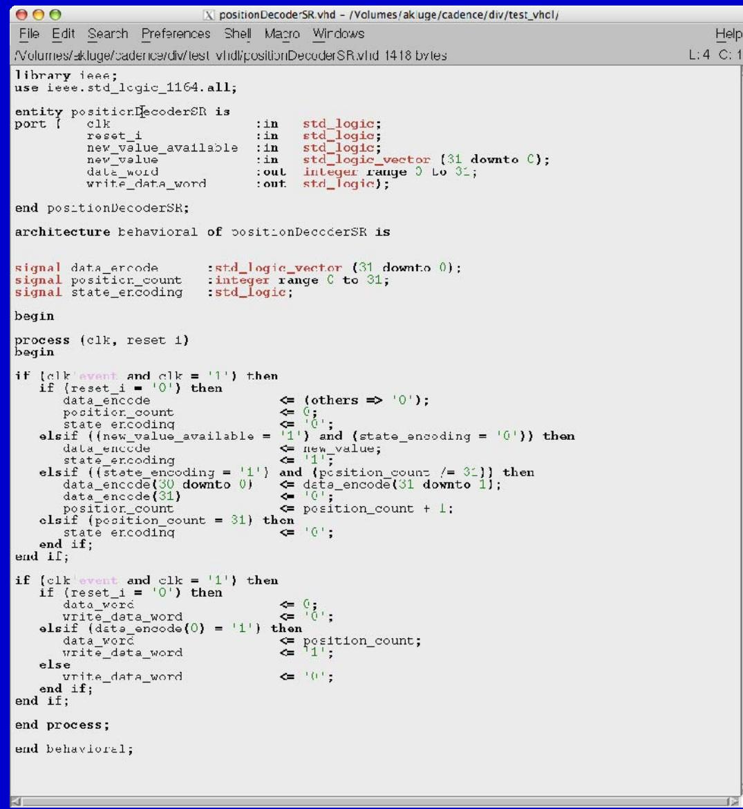
A screenshot of a Cadence VHDL editor window titled "positionDecoderSR.vhd - /Volumes/akluge/cadence/div/test\_vhdl". The window displays VHDL code for a "positionDecoderSR" entity. The code defines inputs and outputs, an architecture, and a process block with multiple conditional statements (if-else) for handling data encoding and decoding based on clock edges and reset signals.
