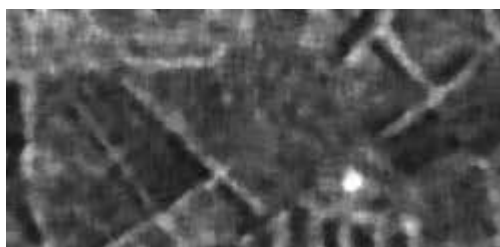
Speckle reduction using an averaging filter
