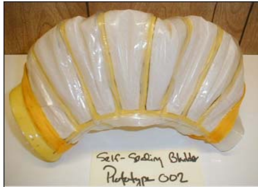
Figure 17. Self-healing Viscoelastic Gel Localized on Each Pattern Piece of SSA Lower Arm Bladder
