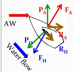
Component of the forces perpendicular to flow
