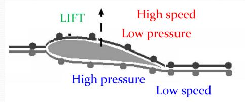
Top of the airfoil is shaped to provide longer path than bottom.
