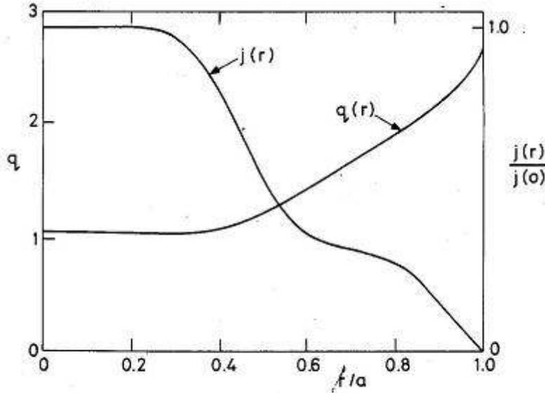
Fig 4 current profile stable to tearing modes
