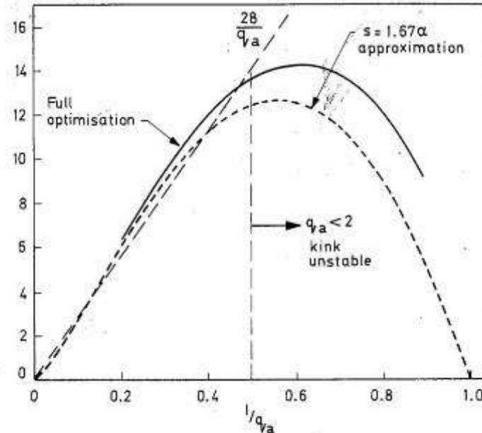
Fig 3 Max.  $\beta$  as a function of  $q_a$
