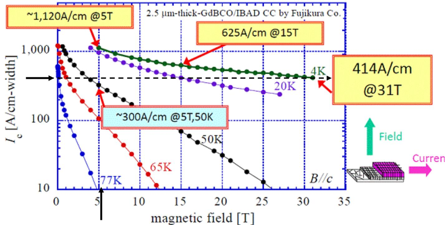
Example 1: moving vertically, in a field of 5T HTS tape can transmit 10A at 77K, but 300A at 50K and 1100A at 4K
