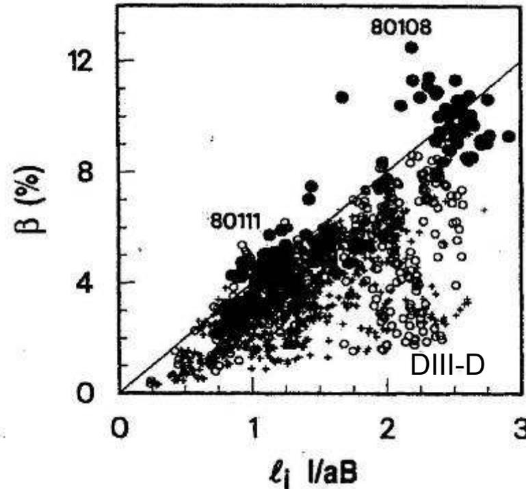
Internal inductance  $l_i$  is small for flat current profiles, large for peaked ones. Although increasing peakedness can raise  $\beta$  it has many confusing effects...
