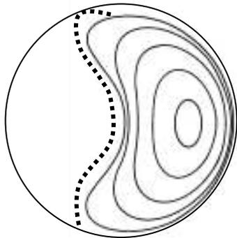
**Reason 1:** If for this high-beta plasma in a circle section tokamak,  $\langle \beta \rangle$  is evaluated over the bean-shaped (dashed) area, a higher value is obtained: for the omitted area contains large  $B^2$  contributions which reduce the circle value.
