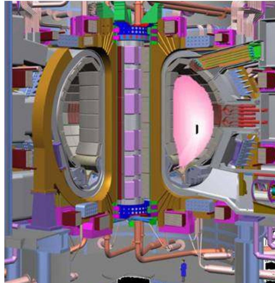
**ITER:** the TF magnet is LTS ( $Nb_3Sn$ ) in steel casing. It uses a small part of the central stack. There is a large central solenoid to power long pulses. The LTS conductor max field is 11.8T; field at  $R_o$  (6.2m) = 5.3T
