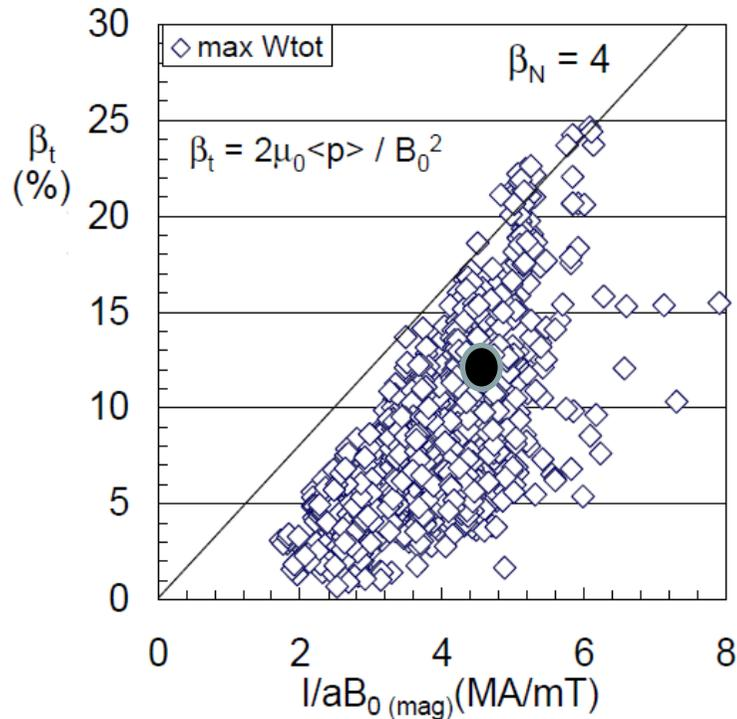
At any point, it may be possible to increase  $\beta$  by increasing li PROVIDED sawteeth or internal modes or tearing modes are not destabilised, and the edge q value does not become close to 2, 3, etc...
