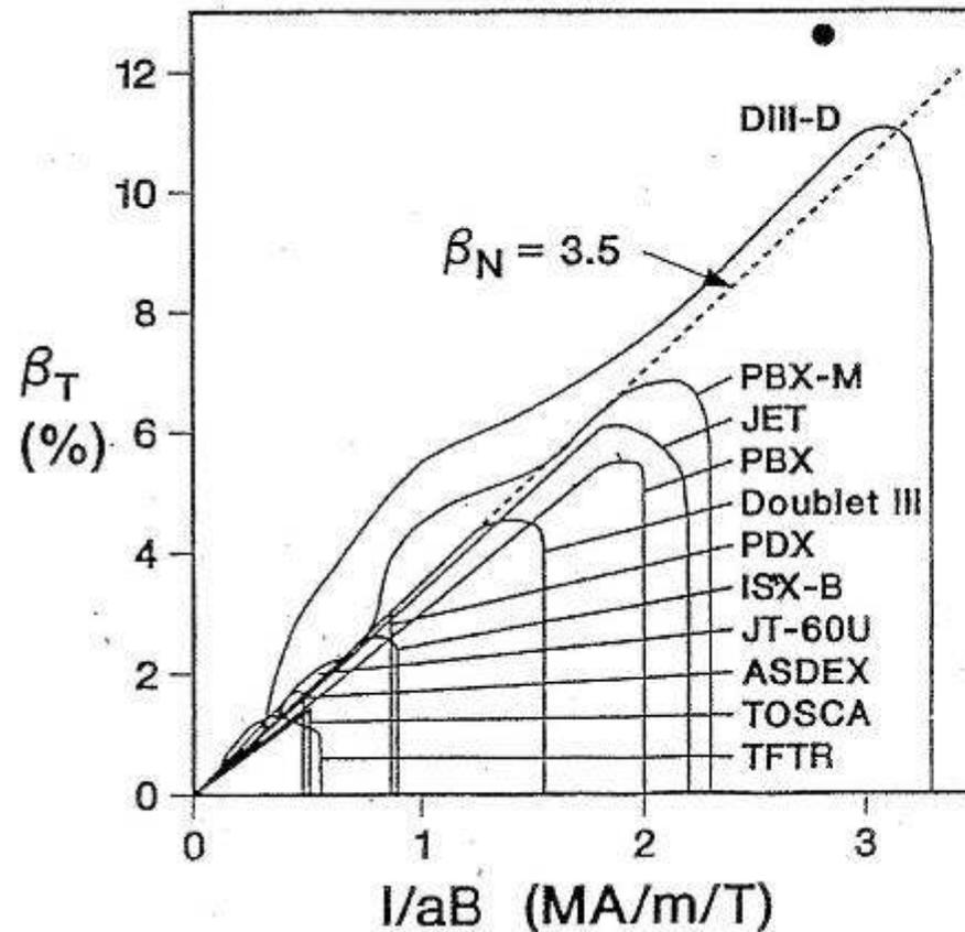
For each tokamak, the right-hand limit to operation is the onset of the low- $q$  limit at  $q_a \sim 2$
