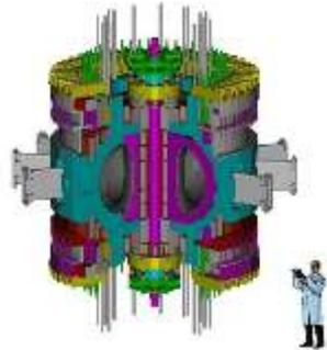
**IGNITOR:** The TF magnet is copper. It is designed to give the max possible field for short pulses. The field at the edge of the copper is 20T, field at  $R_o$  (1.3m) = 13T.
