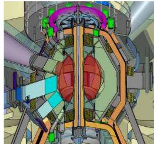
To produce  $B_T = 2.5T$  at  $R_o = 0.85m$  requires c/stack current of 10.5MA; to power the TF and PF coils requires 220MW (dissipation being high in copper coils); costing (assuming 1kWh costs 10p, and 50% operation), **£1.6B per year.**
