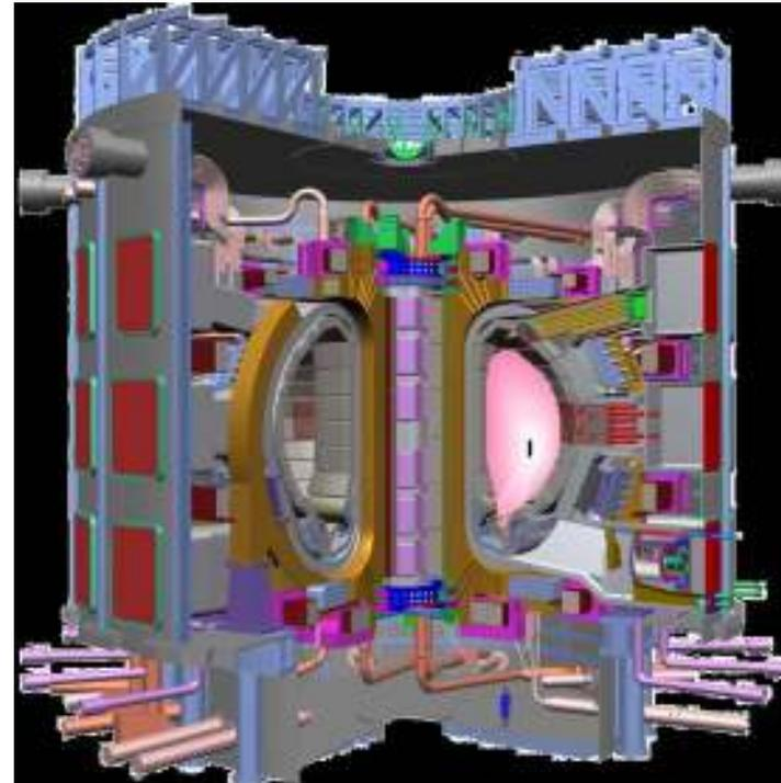
The large volume of ITER increases the confinement time; and the high  $I$  and  $B$  help contain the charged  $^4\text{He}$  particles, which further heat the plasma
