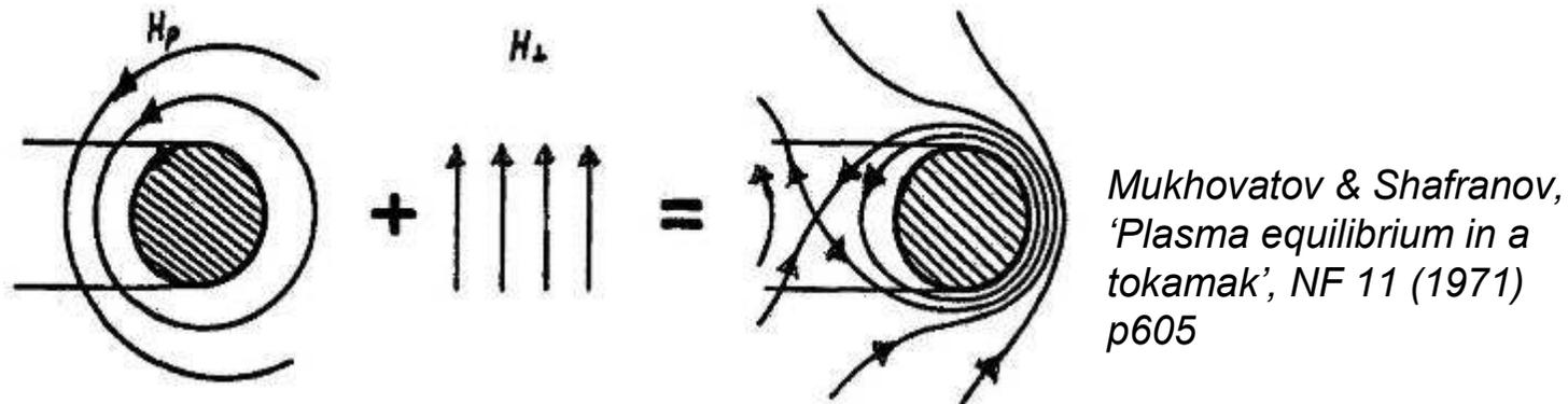
Plasma column (current out of paper) needs vertical field to provide equilibrium; as pressure (beta) increases more vertical field is required to hold plasma
