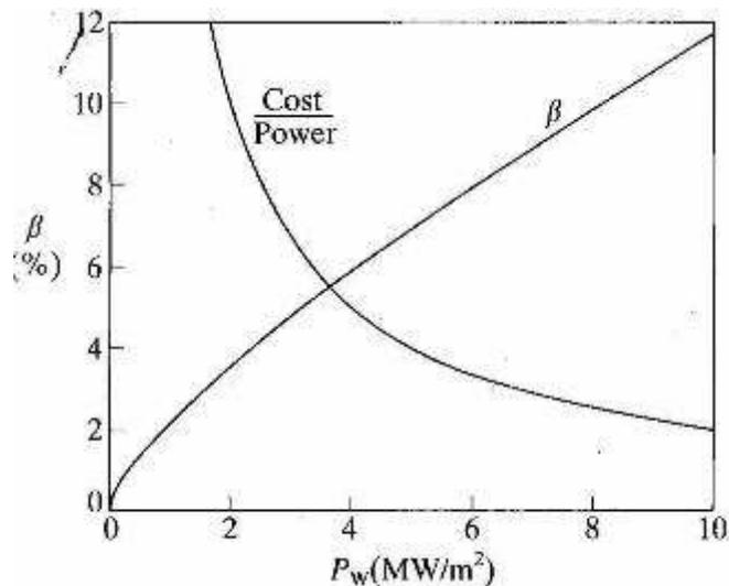
For a typical fusion reactor, build cost /power reduces as wall load increases (and  $\beta$  increases). Limits imposed by damage to wall at high  $P_w$ , and/or instabilities at high  $\beta$  (from Wesson, Tokamaks, 1987)
