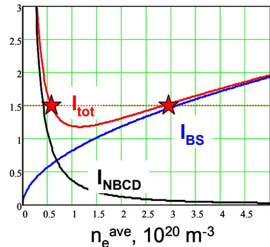
*Density dependence of **NBCD**, **bootstrap** current and total non-inductive current for  $P_{NB} = 6$  MW, 130keV and H-factor  $H = 1.4$ . Stars show two possible operating points.*
