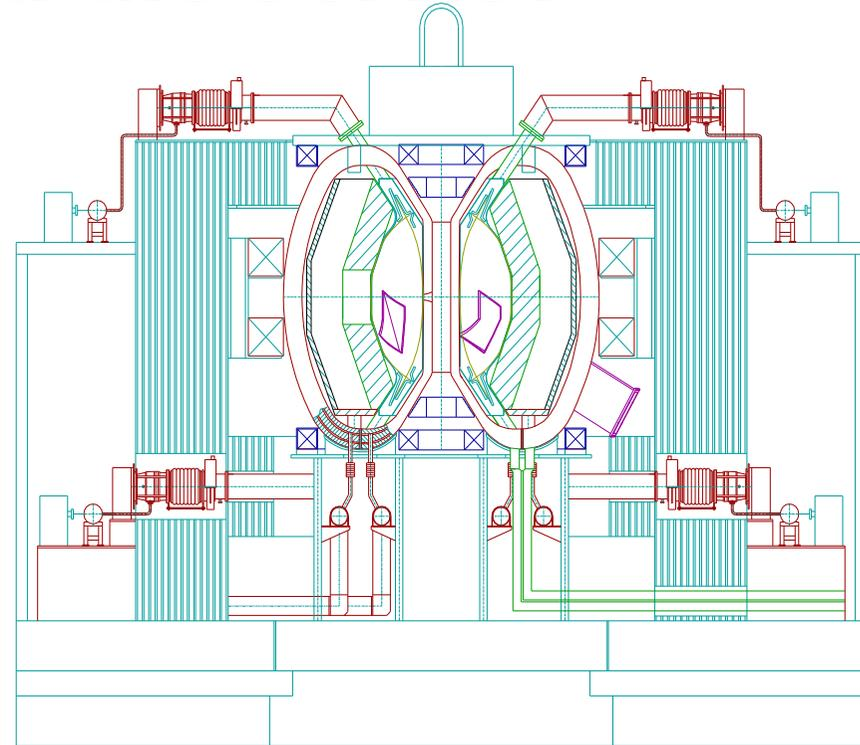
Both VV and TFC are changed after reaching the fluence limit or in a case of accident
