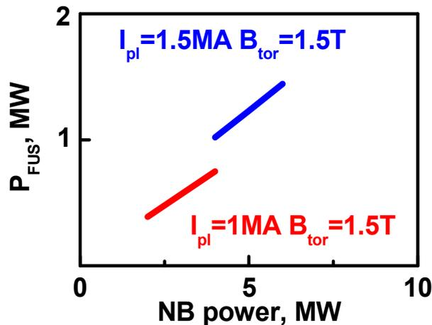
*Fusion output in the SCFNS vs injected power at 130keV with D/T 50/50 mixture in steady-state for plasma current 1 MA (red) and 1.5 MA (blue),  $n_e^{ave} = 10^{20} m^{-3}$*
