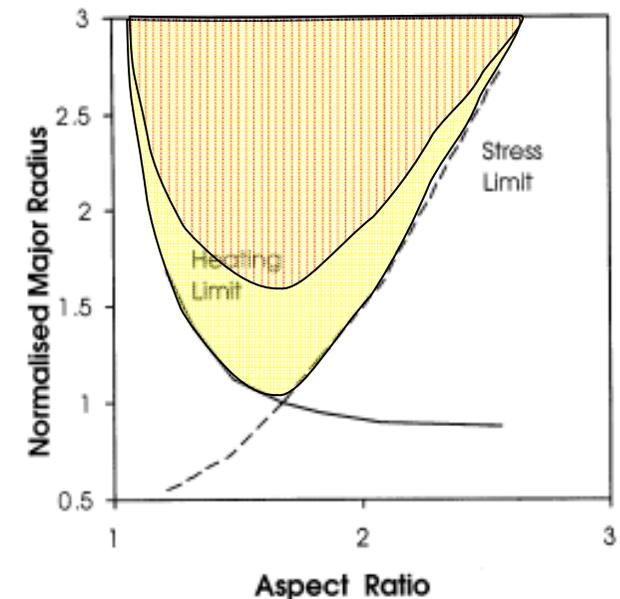
*Normalised (on R=0.57m) device size as a function of aspect ratio at fixed neutron wall load,  $\beta_N$  and  $q_c=3$*
