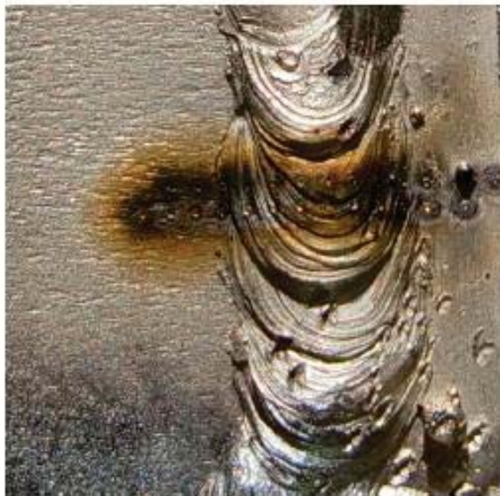
(a) A metal sample with welded bump (~ 1.5 mm height) .
