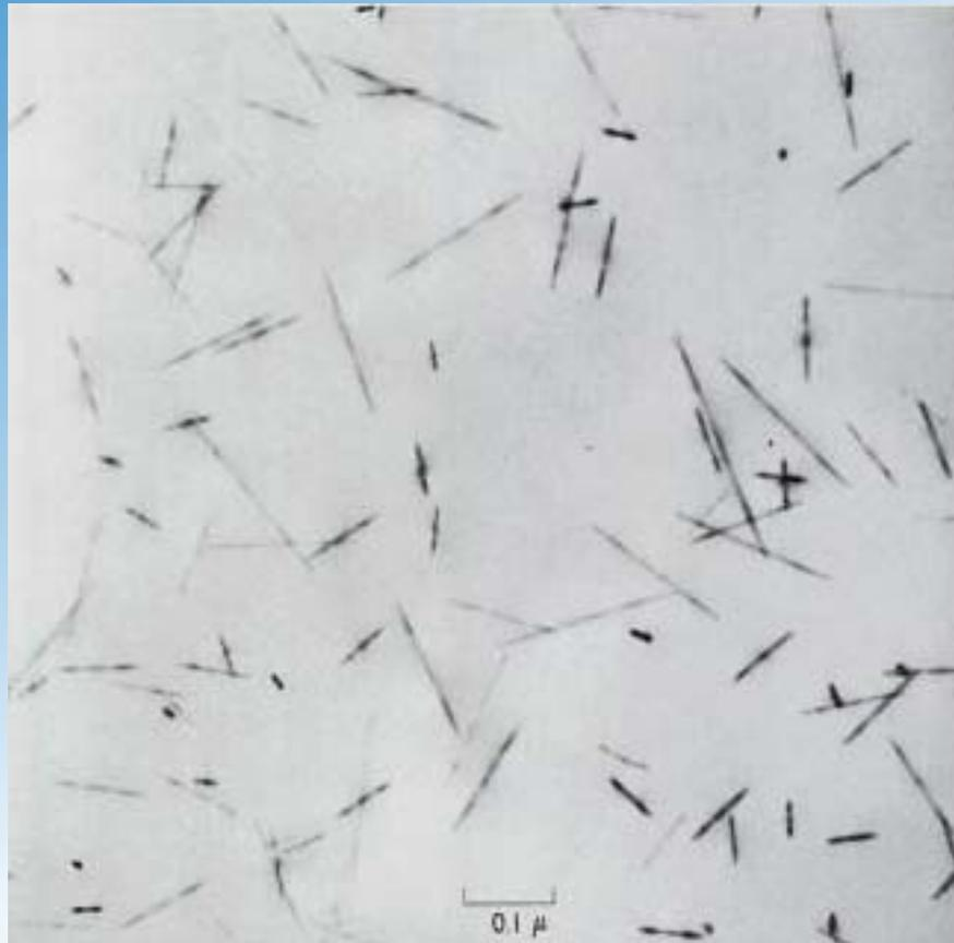
TEM image of tracks from  $^{235}\text{U}$  fission fragments in a synthetic fluor-phlogopite mica.
