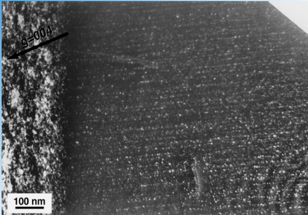
**Microstructure beyond the end of range of the 2 MeV Al ion pre-irradiated region in spinel after 430 MeV Kr ion irradiation**
